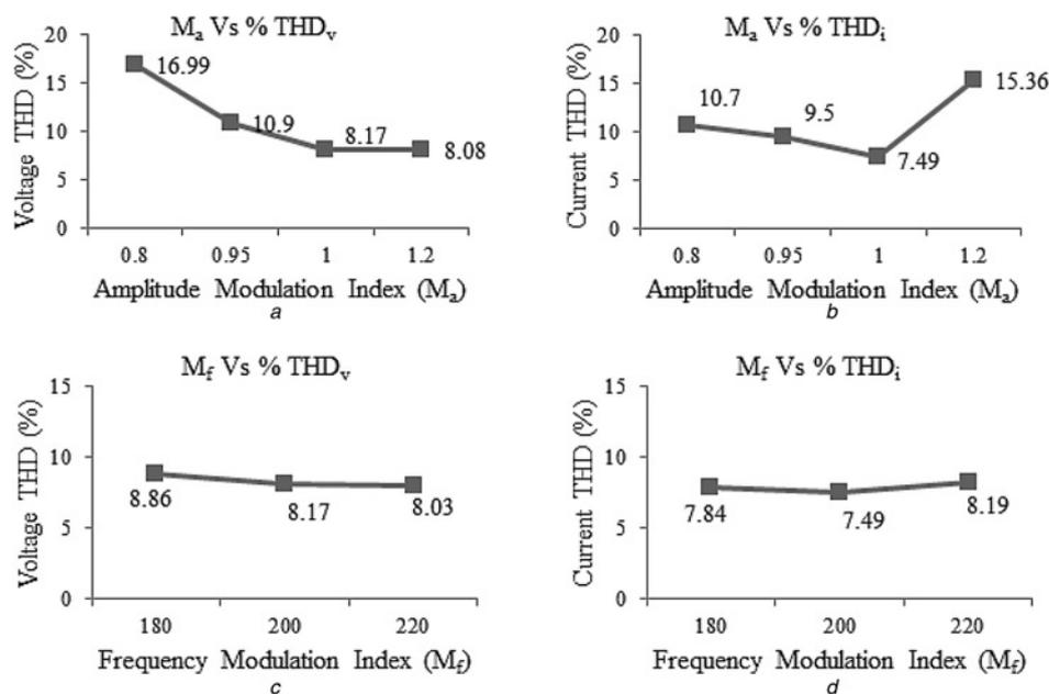
Fig. 6 Voltage and current THD analysis (for motor drive system,  $V_m = 325 \text{ V}$ )
