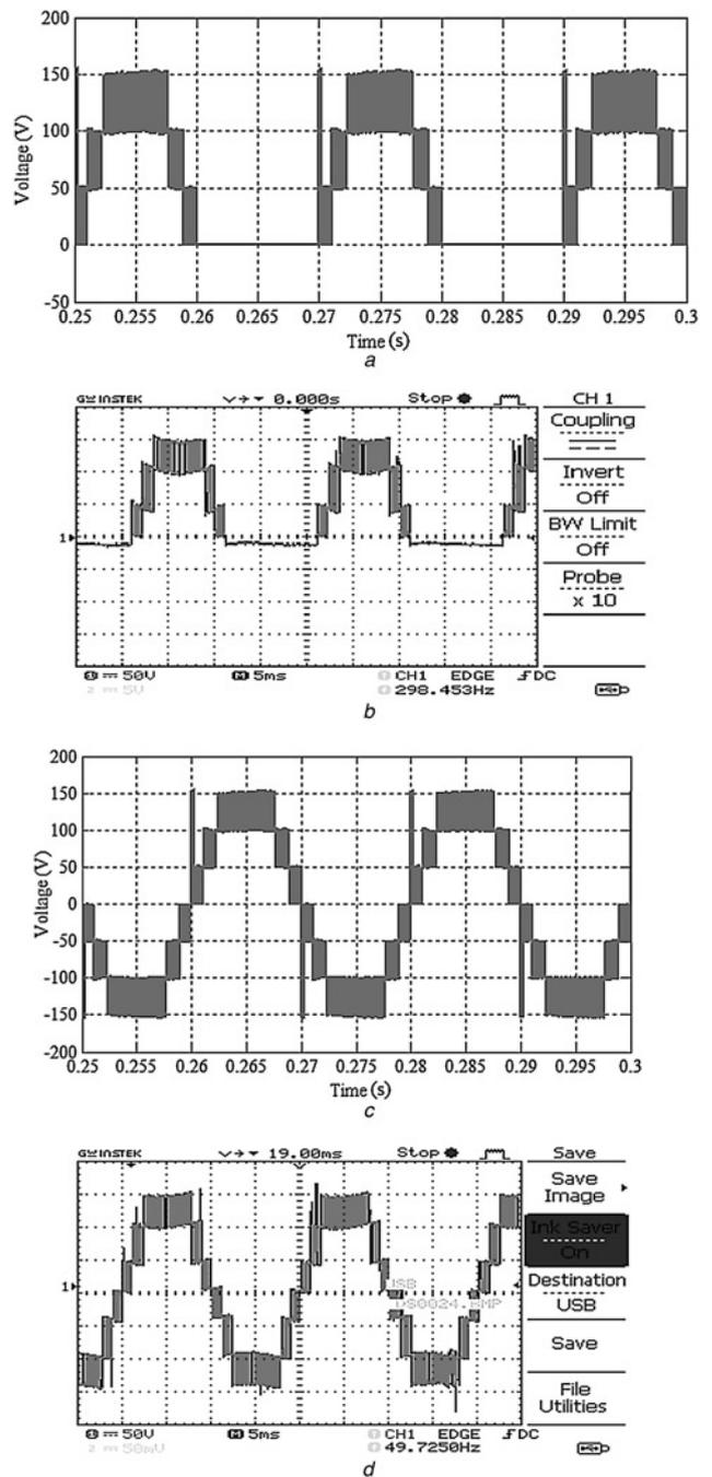
**Fig. 8** Voltage across the H-bridge inverter switches  $S_3$ ,  $S_4$  and load
