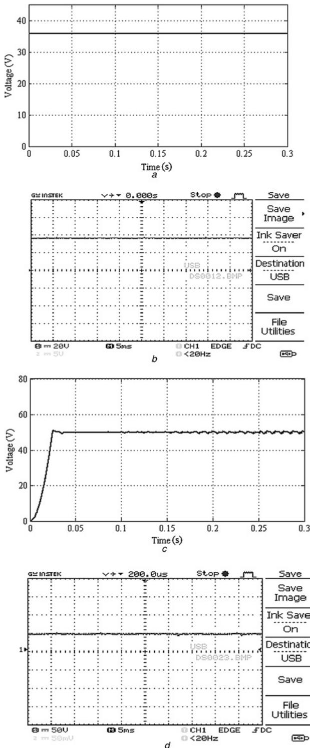
**Fig. 7** Input and Output Voltage of Boost Chopper I
