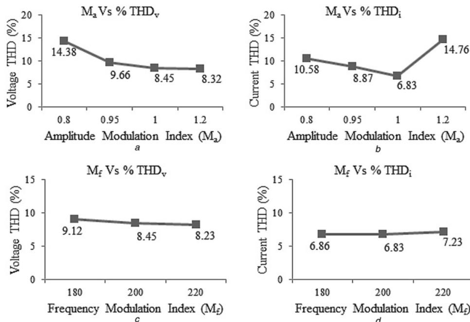
**Fig. 9** Voltage and current THD analysis (for motor drive system,  $V_m = 150$  V)
