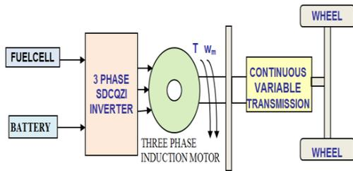
Fig.1. Block Diagram of Hybrid electric vehicle with proposed SDCqZSI.
