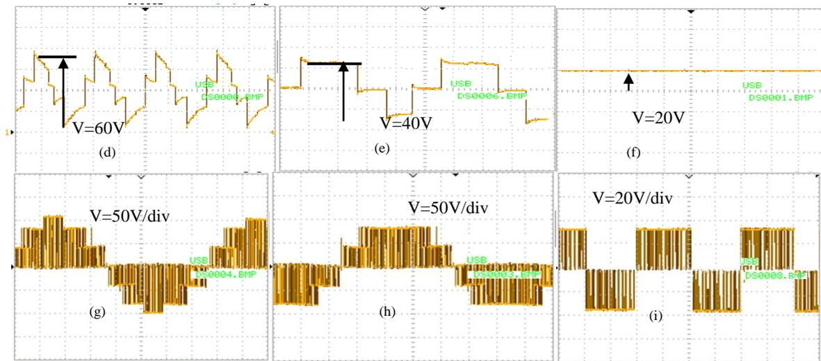
Fig . 11. Hardware output of gate pulse for stepped DC link circuit(a) S1, (b) S2, (c) S3, (d)  $V_{sdC}$  for three sources, (e)  $V_{sdC}$  for two sources, (f)  $V_{sdC}$  for single source, (g)  $V_{ac}$  for  $V_{sdC}=60V$ , (g)  $V_{ac}$  for  $V_{sdC}=40V$ , (g)  $V_{ac}$  for  $V_{sdC}=20V$  at  $M_a=0.82$
