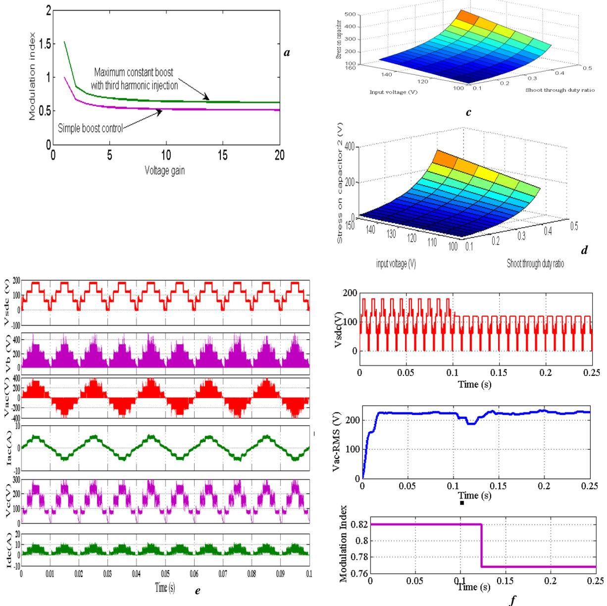
Fig . 7. Simulation response of SDCqZSI (a) Comparison of control techniques, (b)Effect of shoot through duty ratio on boosted DC link voltage, (c), (d) Effect of shoot through duty ratio on capacitor voltages, (e) Response at various stages of Inverter, (f) Control of output voltage by varying  $M_a$
