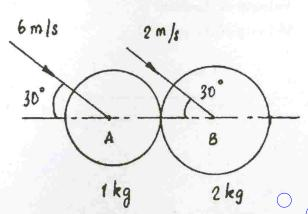
If the coefficient of restitution is 0.5, find the velocity and the direction of the two balls after impact. Also calculate the loss in kinetic energy due to impact and the percentage of loss. (16)
