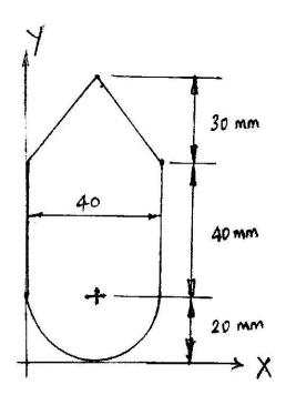
Find the moments of inertia (second moments of area) about both the centroidal axes. (16)
