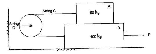
Find the force P required to pull the block B. Also find the tension in the string D. Take coefficient of friction at all contact surfaces as 0.3. (8)
