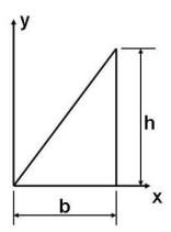
(ii) Locate the centroid of the plane area shown in figure below.
