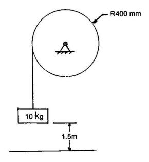
The system starts from rest when the block is at 1.5 m above the floor. Determine the mass of the drum which will allow the block to hit the floor at  $1/4^{th}$  the speed it would have attained if the block alone were simply dropped from the same height. (16)
