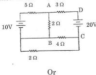
(b) A loud Speaker is connected across the terminals A and B of the network shown in figure below. What should be the value of impedance of the speaker to obtain maximum power transferred to it and what is the maximum power? (13)
