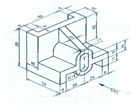
All Dimensions are in mm (OR) 14. Draw the isometric view of the given orthographic views.
