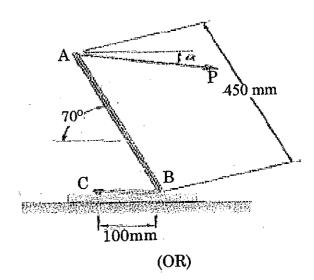
b) Knowing that P = 210 N, replace the three couples with a single equivalent couple, specifying its magnitude and the direction of its axis. (13)
