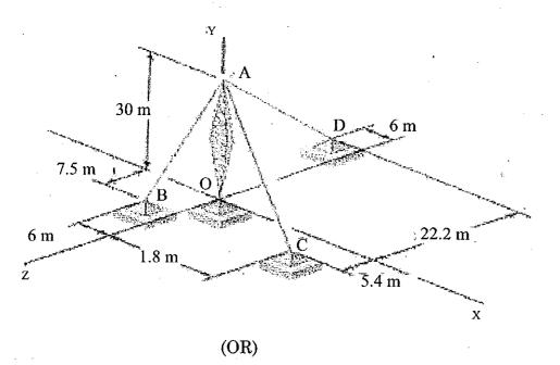
b) Knowing that the tension is 1020 N in cable AB and 850 N in cable AC, determine the magnitude and direction of the resultant of the forces exerted at A by the two cables.
