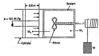
The piston is frictionless, and it is held down against the fluid due to atmospheric pressure of 101.3 kPa. The stirring device is turned 9500 revolutions with an average torque against the fluid of 1.25 Nm. Meanwhile the piston of 0.65 m diameter moves out 0.6 m. Find the network transfer for the system.
