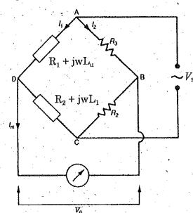
$V_s = 10 \text{ V}_{r.m.s.}, L_1 = 20 \text{ mH}, R_2 = 100 \Omega, R_3 = 100 \Omega$
