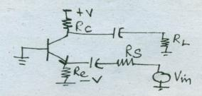
(ii) Identify the feedback topology. Find the open and closed loop gain of the circuit given. Assume  $hie_1 = hie_2 = 2K$ ,  $hfe_1 = hef_2 = 100$ . (10)
