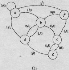
Analyze the Mealy model asynchronous sequential circuit of the following (b) figure and show its stable state and corresponding outputs. Also give its state diagram. (16)
