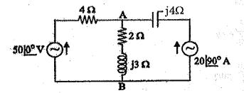
ii) Determine the Thevenin's equivalent across AB for the given circuit. (8)
