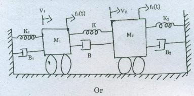
(b) Obtain the transfer function using Mason's Gain formula for the system given. (16)
