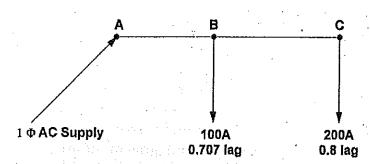
The load resistance and reactance of the distributor are  $0.2\,\Omega$  and  $0.1\,\Omega$  per km respectively. Calculate the total voltage drop in the distributor.
