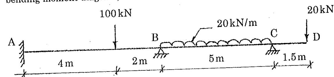
15. a) Analyse the continuous beam as shown in fig. by moment distribution method.
