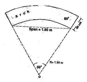
ii) Work out the Brick work and cement plaster to soffit of an arch as per data given below.
