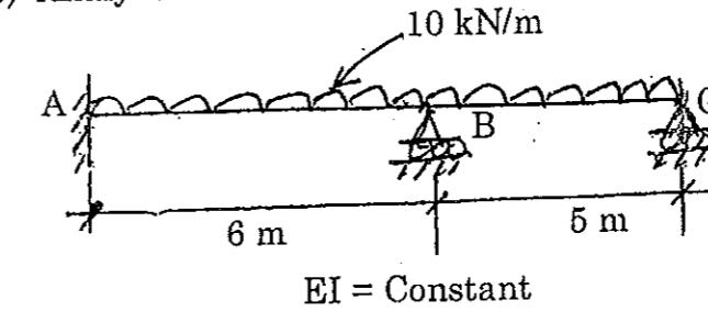
15. a) Analyse the beam ABC shown in Fig. Q 15 (a) by stiffness method.
