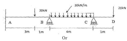
(b) Analyse the frame by moment distribution method.
