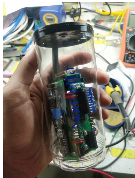
3D Printed Compact CanSat (Vertical Stacking of Boards Around Battery) (Patents Filed)
