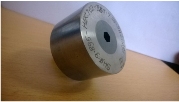
Fig. 20 Specially machined extrusion die with cosine profile
