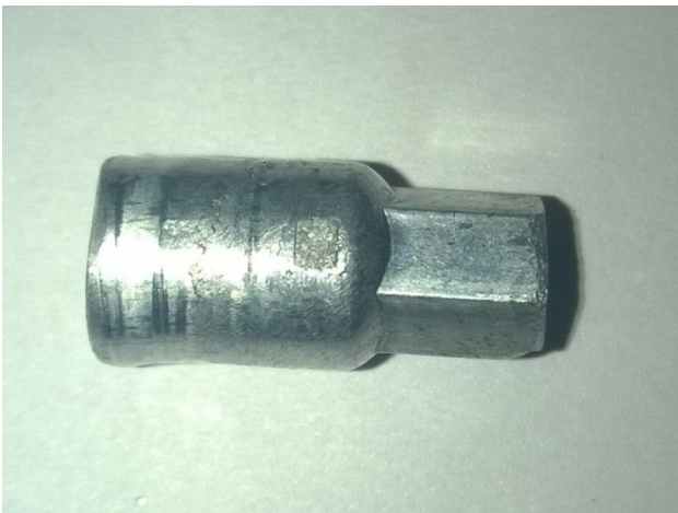
Fig. 21 Extruded hexagonal section
