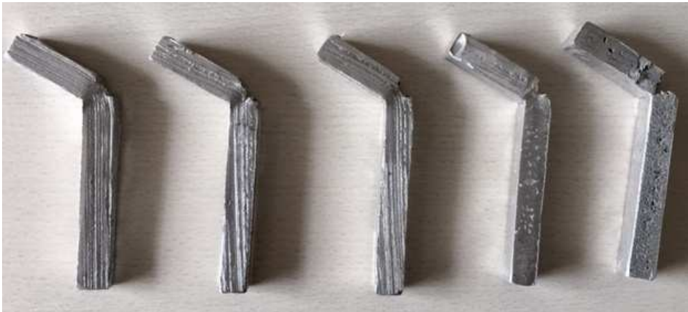
Fig 9. Fractured impact composite specimen
