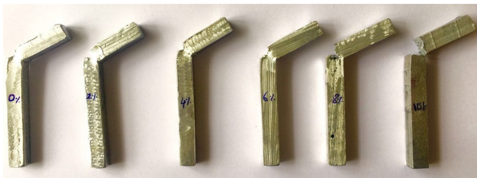
Fig. 14. Fractured Izod impact test specimen.
