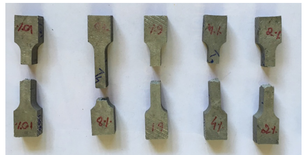
Fig. 9. Fractured tensile test specimen.
