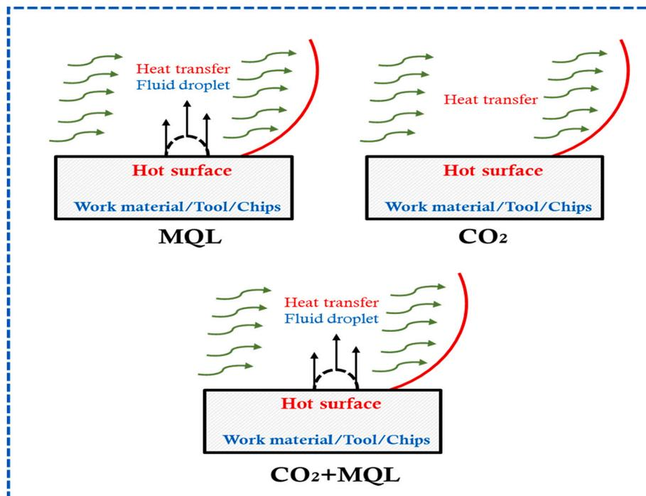
Fig. 3. Distinct cutting environments in milling of Nimonic 80A.
