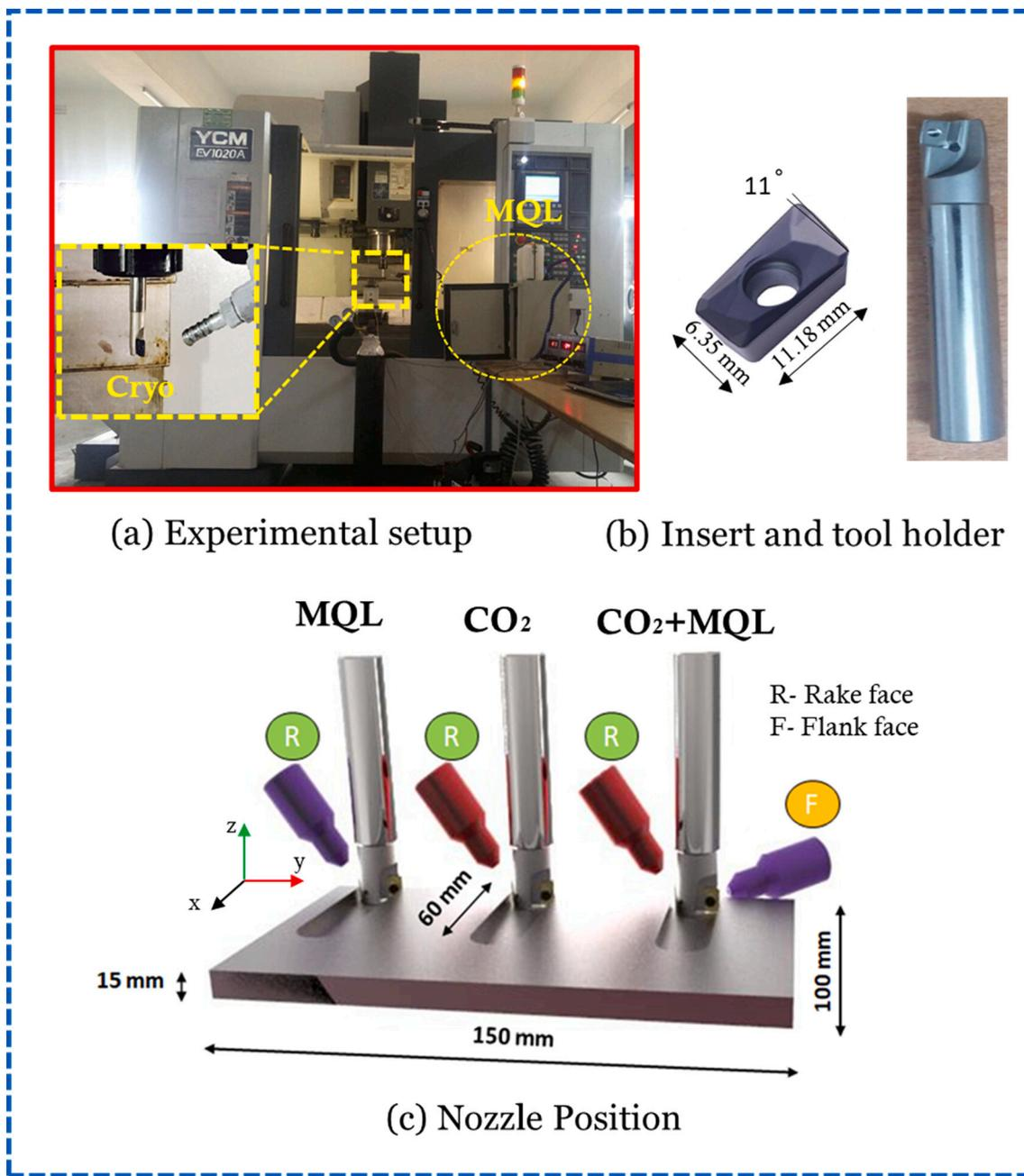
Fig. 1. Experimental methodology (a) Experimental Setup, (b) Insert and holder (c) Nozzle positions for MQL and Cryogenic system.
