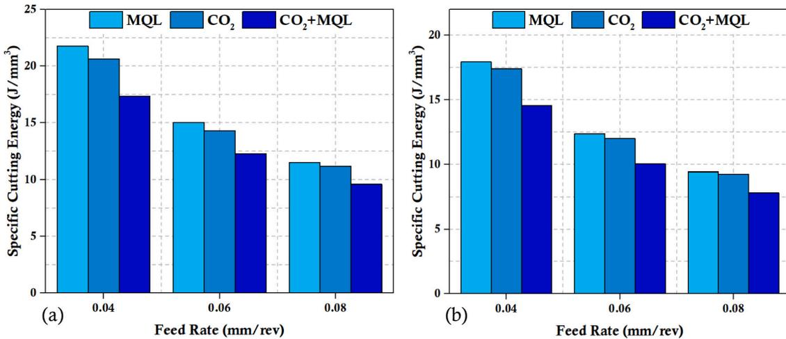
Fig. 6. Impact of distinct environments and speed-feed combo on Specific cutting energy at a Vc of (a) 75 m/min (b) 90 m/min.
