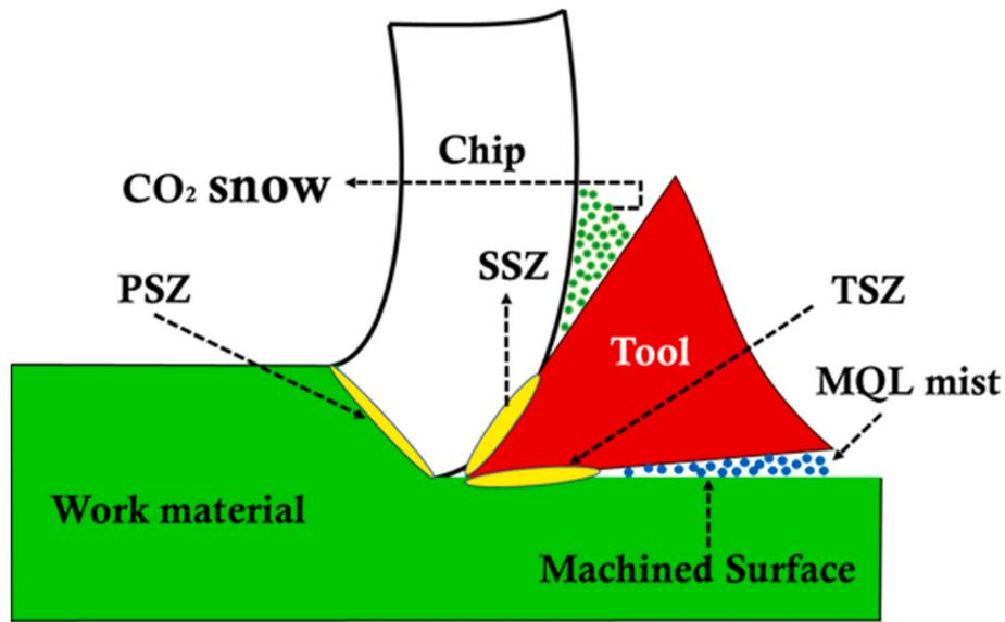
Fig. 2. Effect of shear zones under hybrid metal cutting.
