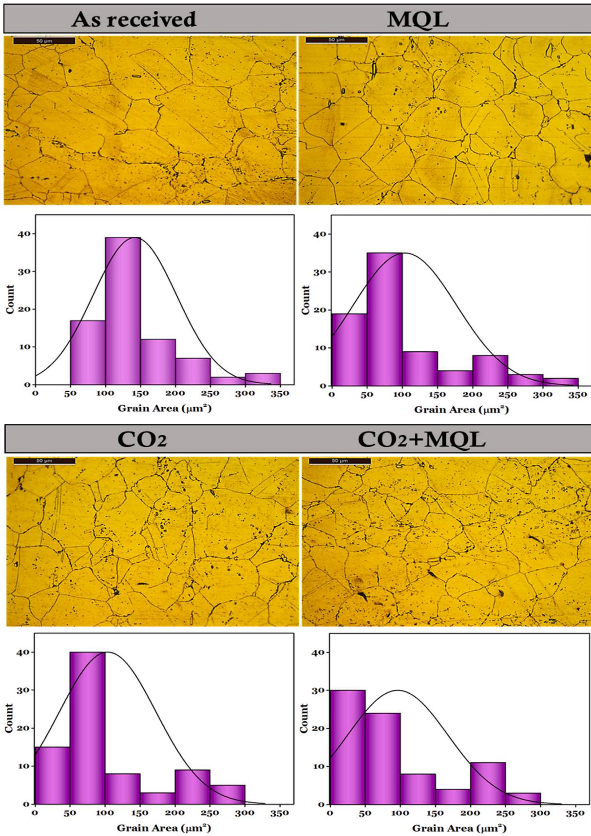
Fig. 9. Histogram of grain size distribution under distinct environments at  $V_c = 90$  m/min and  $f = 0.08$  mm/rev.
