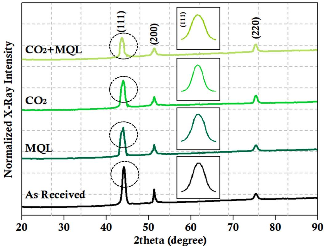
Fig. 8. X-ray diffraction of Nimonic-80A alloy under distinct environments at  $V_c = 90$  m/min,  $f = 0.08$  mm/rev.
