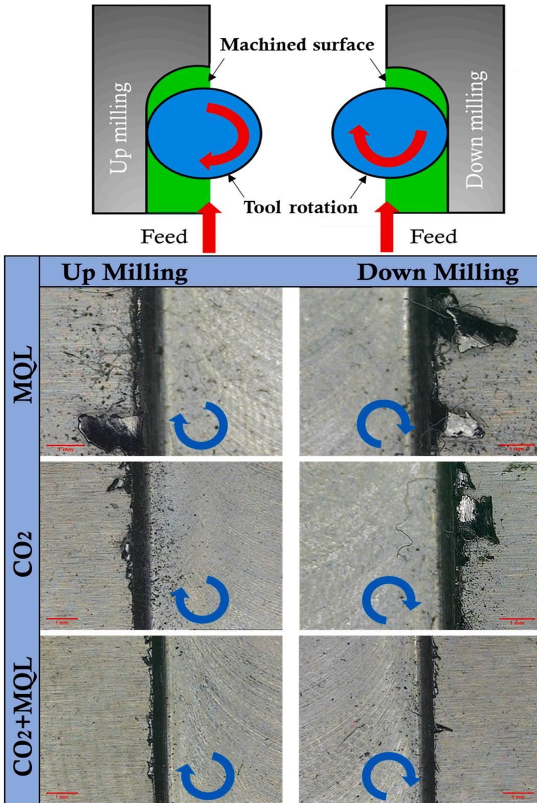
Fig. 7. Development of Burr under distinct environments at  $V_c = 90$  m/min,  $f = 0.08$  mm/rev.
