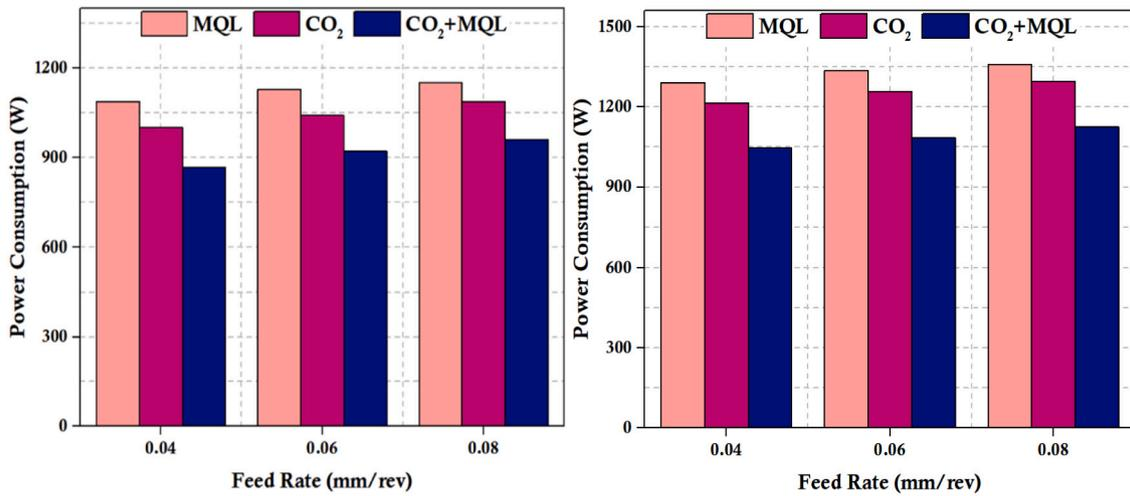
Fig. 5. Impact of distinct environments and speed-feed combo on power consumption at a Vc of (a) 75 m/min (b) 90 m/min.
